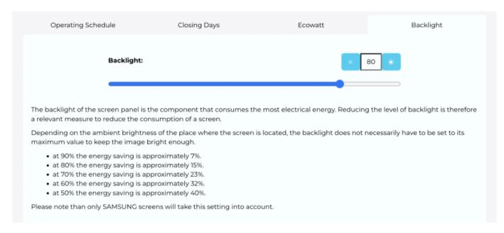
The backlight of the screen is the component that consumes the most energy (between 80% and 95% of its consumption). Reducing the level of backlighting is therefore an effective measure to reduce the power consumption of a display.
