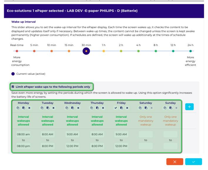
If this parameter is changed while the screen is in standby, the modification will only take effect at the next wake-up.
