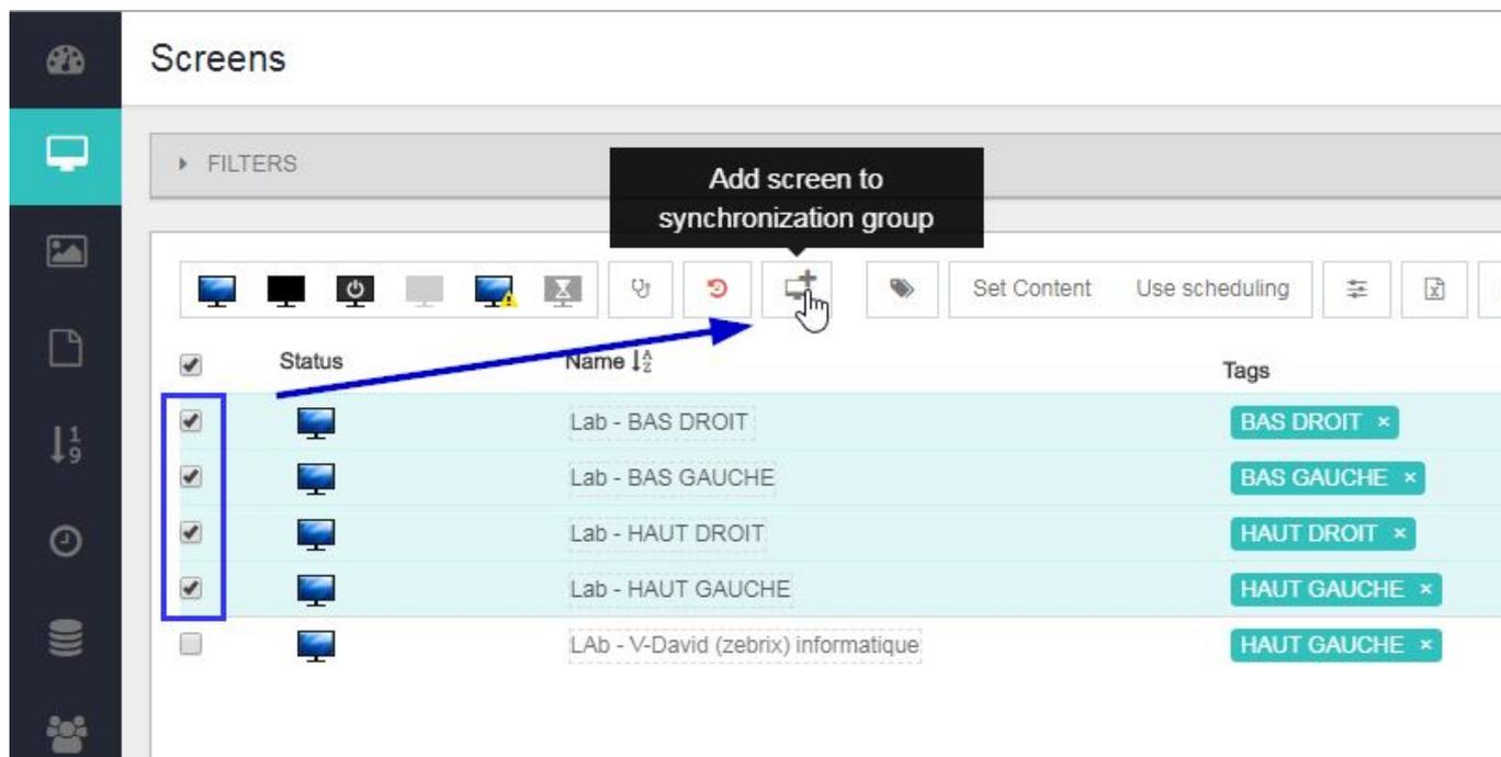
The screenshot shows the 'Screens' management interface. At the top, there is a 'FILTERS' section. Below it is a toolbar with various icons, including a plus sign icon for adding screens. A callout box labeled 'Add screen to synchronization group' points to this icon. Below the toolbar is a table with columns for 'Status', 'Name', and 'Tags'. The first four rows are highlighted with a blue box, and a blue arrow points from this box to the plus icon in the toolbar.
